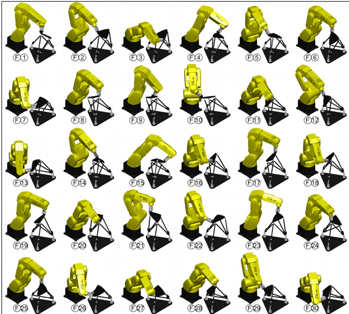
Figure 4.6 Robot configurations used for calibration (continues)
