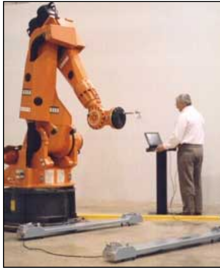
Figure 1.1 Robot calibration using the CompuGauge device 1
