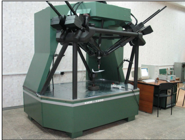
Figure 3.1 A CMM of hexapod design (courtesy of Lopic, Russian Federation)
