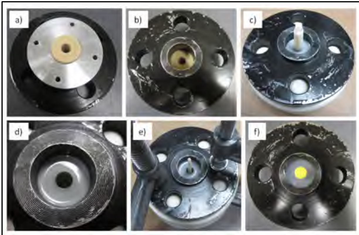
Figure 5.3: Summarizing overview of the development process of the artificial external ear model. a) Back view: Polyurethane cylinder, to mimic bony tissue, (beige) is press-fitted into slip-on flange (black). Anterior disc of excitation cage is press-fitted around bony tissue b) Front view: Polyurethane cylinder after press-fitting into slip-on flange. Remaining volume of central bore hole in slip-on flange to be filled with two different types of silicone to mimic soft and skin tissues. c) Front view: After injection of the first silicone that is used to mimic the soft tissue, the silicone is cured overnight (grey). The insert (white) delimits the soft tissue cylinder and is removed after completion of the curing process. d) Front view: Final result after molding of soft tissue cylinder and removal of the insert. e) Front view: A second insert (white) is placed concentrically in the soft/bony tissue subassembly. Its diameter is chosen so that the second silicone, used to mimic the skin tissue, can fill the remaining volume that corresponds to the ear canal walls and the skin tissue around the ear canal entrance. f) Front view: following the molding and curing of the skin tissue domain, the second ABS insert is removed. An earplug can be inserted into the finalized artificial external ear model
