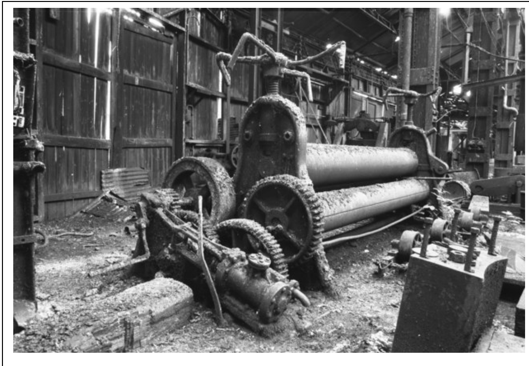
Figure 2.1 The steam-powered roll bending machine (Allen, 1985)
