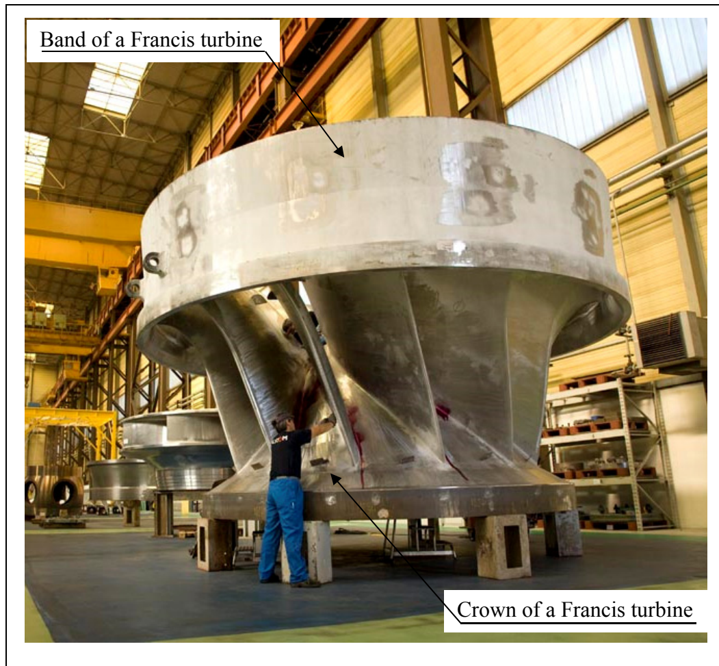
Figure 1.5 Example of Francis turbine runners (Alstom, 2014)
