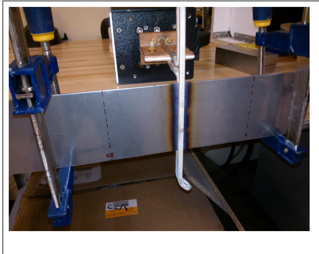
Figure I.3 Heating plate experiment: stationary case
