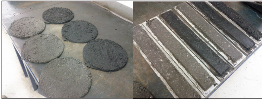
Figure 8.7 Colored and conventional micro-surfacing mixtures prepared for wet track abrasion and loaded wheel tests
