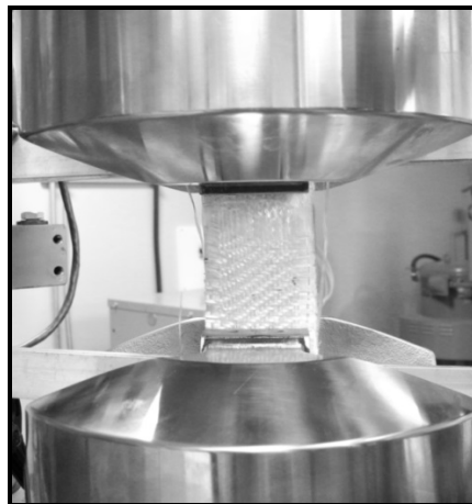
Figure 3.5. A tufted sample clamped for in-plan tension test
