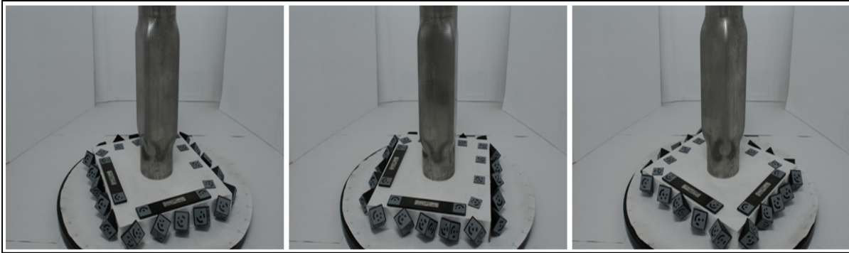
Figure 2.16: Pictures from different views of the deformed tube
