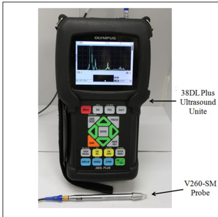
Figure 2.10: The ultrasonic thickness measurement device (38DL Plus)
