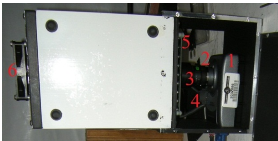
Figure 1.3 Top view of the installed TIS-III NI-1744 Camera (1), Computer M1214-MP lens (2), camera guide bracket (3), camera Light control connector (4), excitation light board (5), cooling fan (6)
