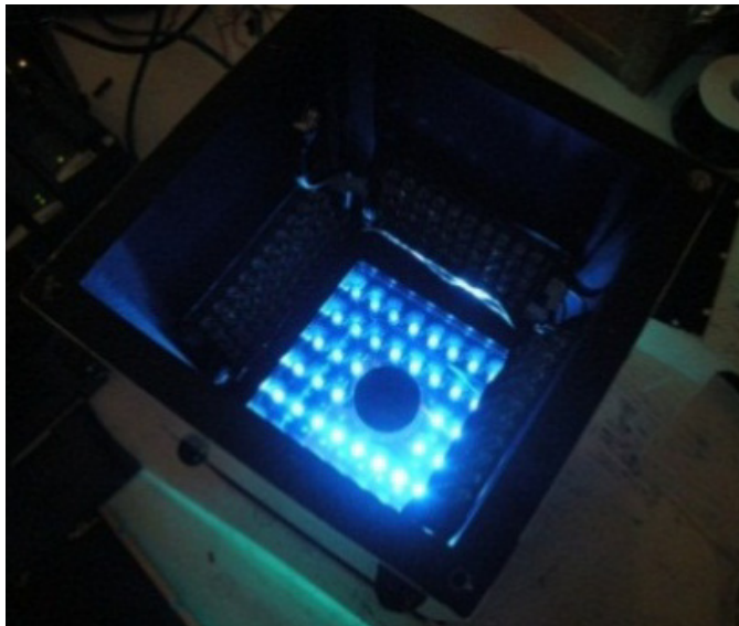
Figure 1.8 TIS-III excitation LEDs behind a band-pass filter
