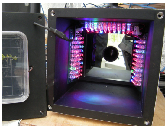
Figure 1.6 Grow lights boards and positioning within the TIS-III
