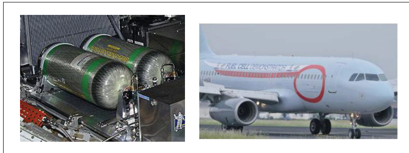
Figure 0.5 Fuel cell emergency power system developed and tested by DLR Adapted from DLR (2010)
