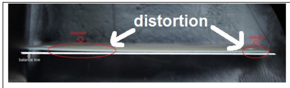
Figure 6.6 Side view of the LTCC fabrication broken in the fabrication process because of very thin thickness
