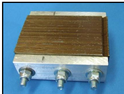
Figure 2.2 Lamination stack used for mechanical abrasion
