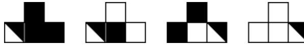
Figure 2.2: Compacted rule table for CA-184. Cells where the state does not matter (logical OR) are split diagonally.
