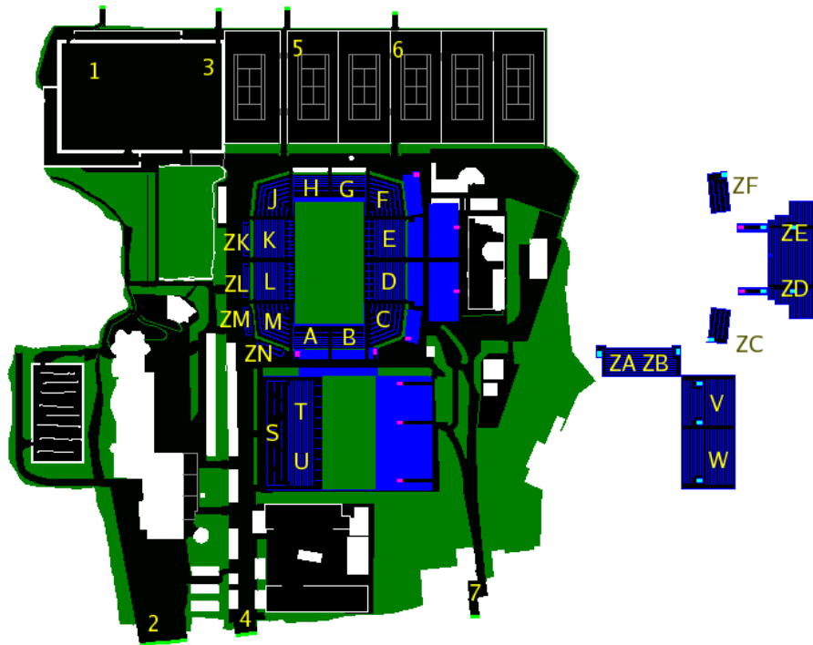
Figure 5.1: Plan of the Rochusclub area with numbers of exits (1-7) and names of grandstands (A-ZF). Higher floors are moved to the right. Black pixels mark free cells, white and dark green walls. Exits are marked light green. Floor exits are drawn cyan and floor entrances magenta.
