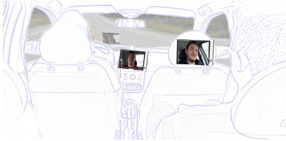
Figure 54. Concept of a driver-passenger video link. Driver gets shown a video image of the rear-seat passenger either on a monitor mounted at the vertical center stack or in a Head-up display. The rear-seat passenger sees on a monitor in front of him a video image from the driver.
