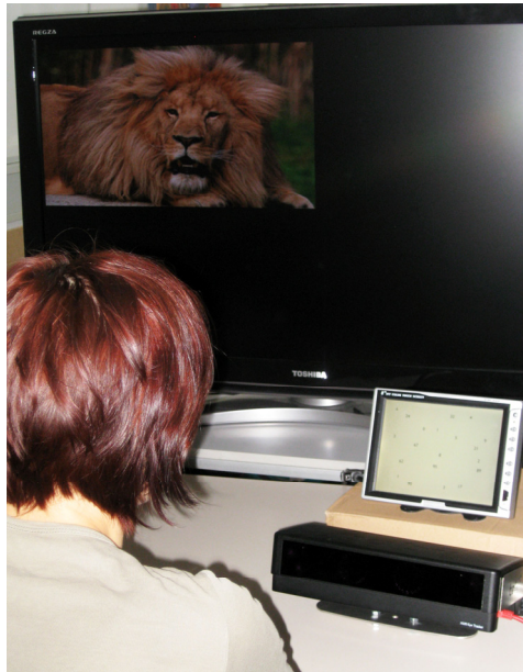
Figure 42. Setup of the fixation study. Participant performs a search task on an 8" display and his attention as grabbed by animal pictures on a 42".
