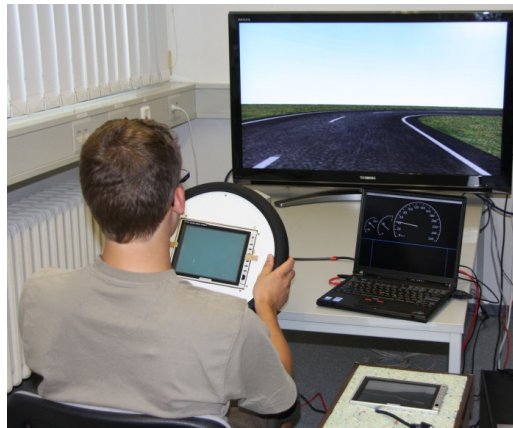
Figure 31. Study setup: Touchscreen displays on the steering wheel and in the horizontal center stack serve as input and output interfaces. Laptop serves as dashboard display (and speedometer). 42" TFT monitor shows first person view of the driving simulator.
