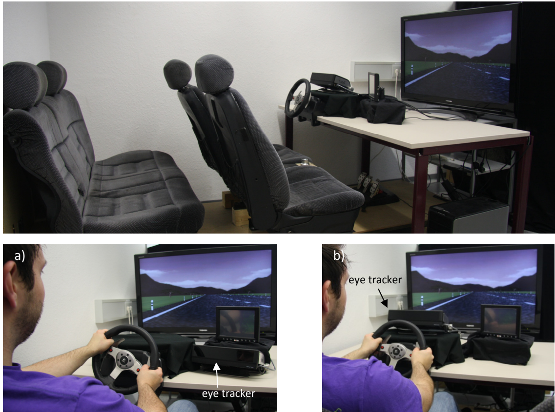
Figure 39. Physical setup of our driving simulator consisting of car seats, a 42" flatscreen, an 8" LCD display, pedals for accelerating and breaking and an eye tracker. a) Eye tracker is placed above the steering wheel in front of the driver. b) Eye tracker is placed underneath the 8" display.
