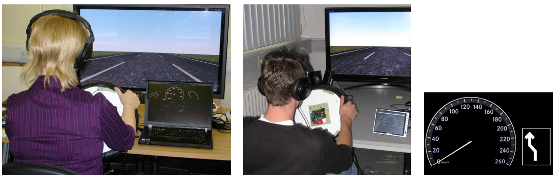
Figure 25. Setup in the first study with the control panel on a laptop (left), setup in the second study with control panel on a 8'' display (middle) and a close-up of the control panel with an direction arrow used in the second study (right).
