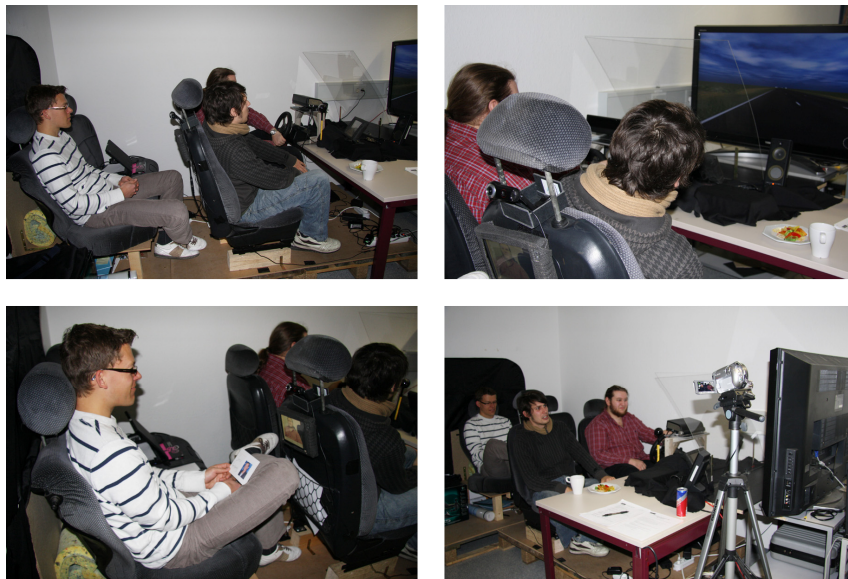
Figure 58. Experimental setup consisting of a 42" screen showing the LCT driving simulation, an 8" screen showing video image of the rear-seat passenger to the driver, another 8" screen showing video image of the driver to the rear seat passenger, an eye tracker, placed above the steering wheel, a webcam facing to the driver, another webcam facing to the rear-seat passenger, a steering wheel and pedals.
