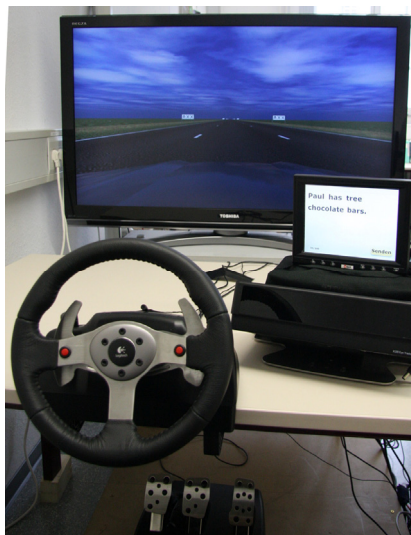
Figure 50. Experimental setup consisting of a 42" screen showing the LCT driving simulation, an 8" screen showing the correction tasks, an eye tracker, a steering wheel with a push-to-select button on the right side and pedals.
