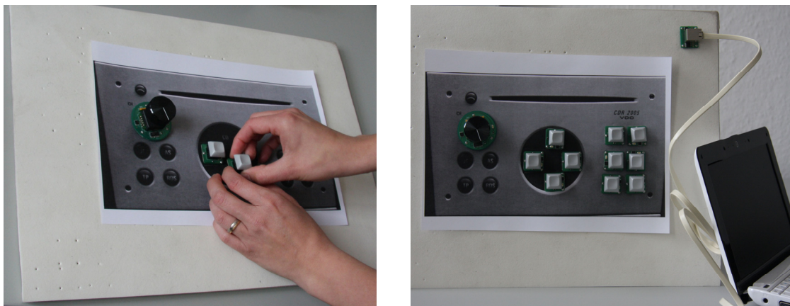
Figure 66. Creating a tangible prototype using VoodooIO [Villar, Gellersen 2007]. The left photographs shows control units being placed on a picture that shows the layout of a radio. On the right side, the completed tangible prototype is shown connected to a netbook.
