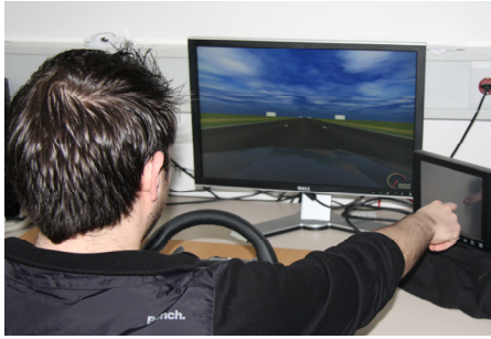
Figure 6. LCT setup consisting of a screen showing LCT driving environment and a gaming steering wheel.
