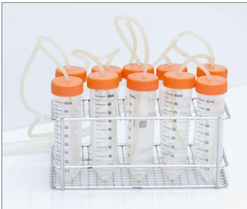
Figure 6: Experimental set-up for analysis of bacterial attachment to pyrite surfaces
