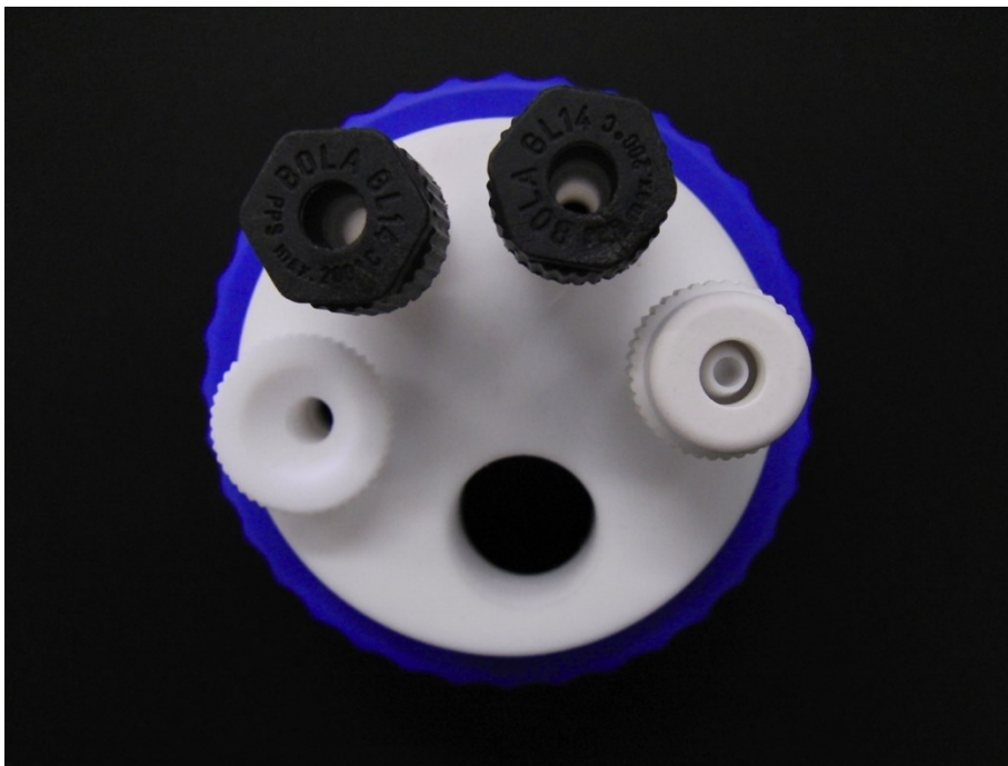
Figure 24: Customised GLS 80 screw cap made out of PTFE with 1•PG 13.5 for a pH electrode, 1•M14•1.5 for the integration of a septum and 3•NTP \frac{1}{4} ” for a cell culture medium inlet and outlet and for gas exchange. [6]
