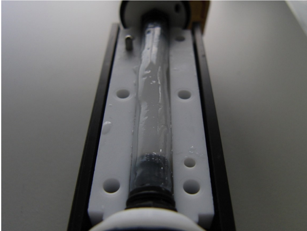
Figure 48: Homogeneously casted fibrin prosthesis with a length of 75 mm in the developed casting mould. [6]
