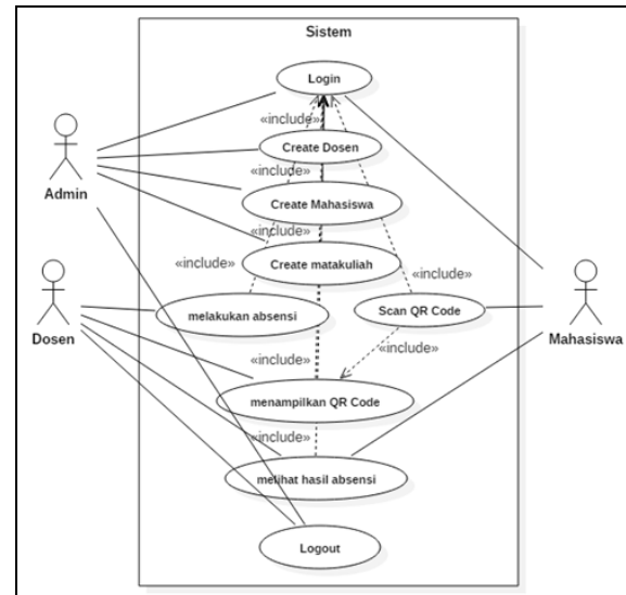
Gambar 3. Use Case Diagram
