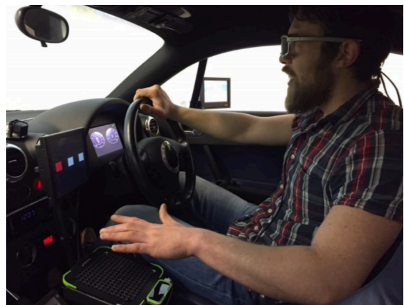
Fig. 8. Ultrasound haptic feedback for in-vehicle interactions [9].
