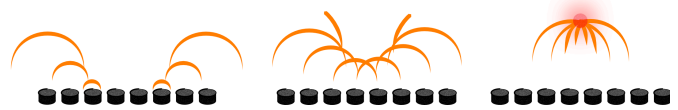
Fig. 1. This image sequence demonstrates the principle of focusing ultrasound from a phased array of eight transducers. The phase of each wave is offset such that they arrive at the desired point at the same time.
