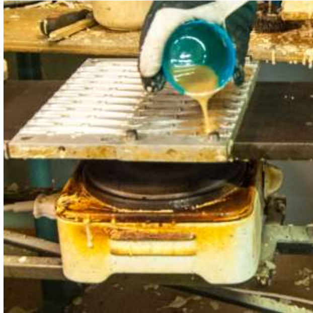
Figure 2. Molding mass poured onto a mold. The hotplate is seen underneath.
