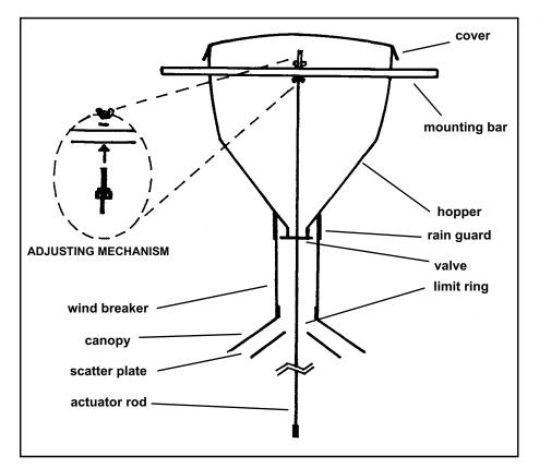
After numerous experimentations for the design of the kinetic feeder, Philip's efforts produced several important and novel improvements. These are the redesign of the valve, addition of a limit ring, addition of scatter plate, addition of wind breaker, optimization of the hopper size, and optimization of the design for transport and storage. A cross sectional view of the kinetic feeder is shown.
