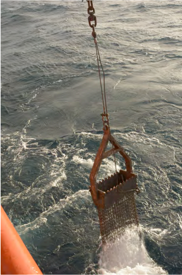
Fig. 6.3 Above: Handling of a chain bag dredge on deck (photo: Kaj Hoernle). Left: The dredge comes back on board after a haul (photo: Roland Knauer).
