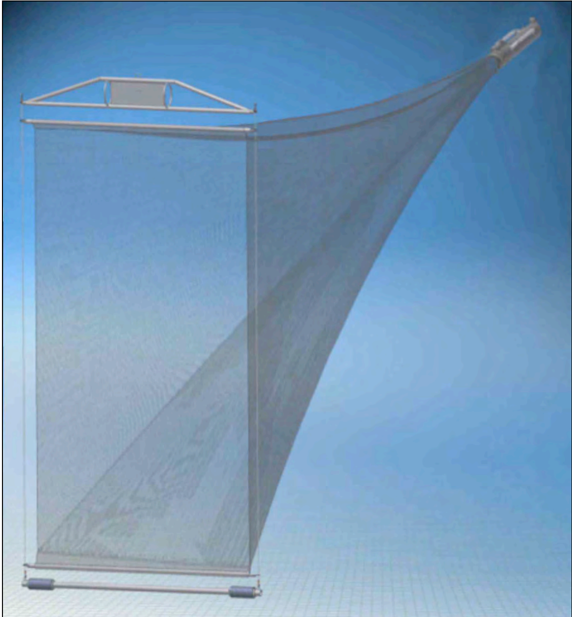
Fig. 7.1: 3D model of the opened RMT-16 trawl net system with closing cod-end.
