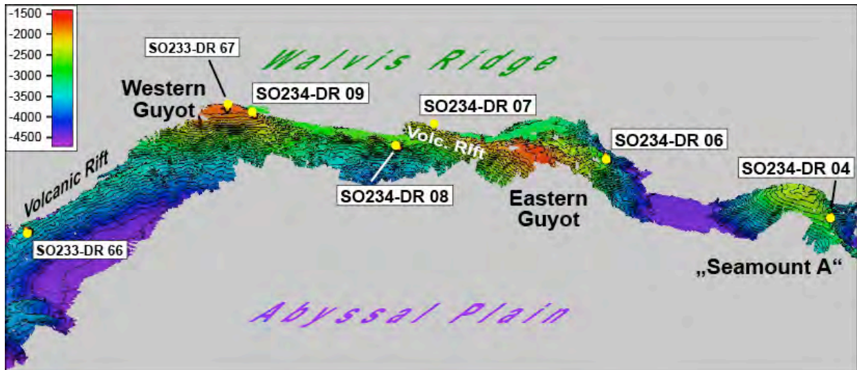
Fig. 6.5: 3D-map showing SO-234/1 and SO-233 mapping and hard rock sampling at the eastern margin of the Walvis Ridge between c. 22° and 22°40' S (view from SE to NW, exaggeration: 3x; interval of contour lines: 100 m). SO-233 and SO-234/1 dredge stations are marked by yellow dots.
