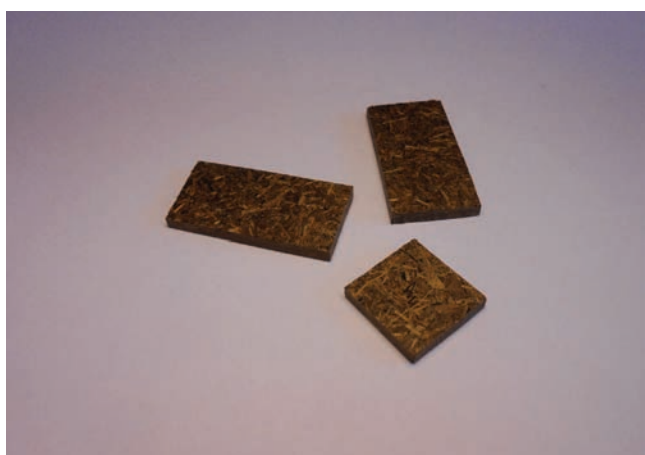
Fig. 6. Photograph of test specimens from fiberboard produced under optimal thermo-pressing conditions.
