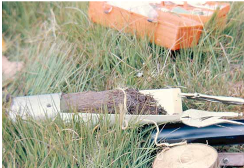
Figure 3. The large-capacity hand corer of Smith et al. (1968). Above: general view of the rig and corer in use; below: plastic liner containing a minimally compressed peat sample.
