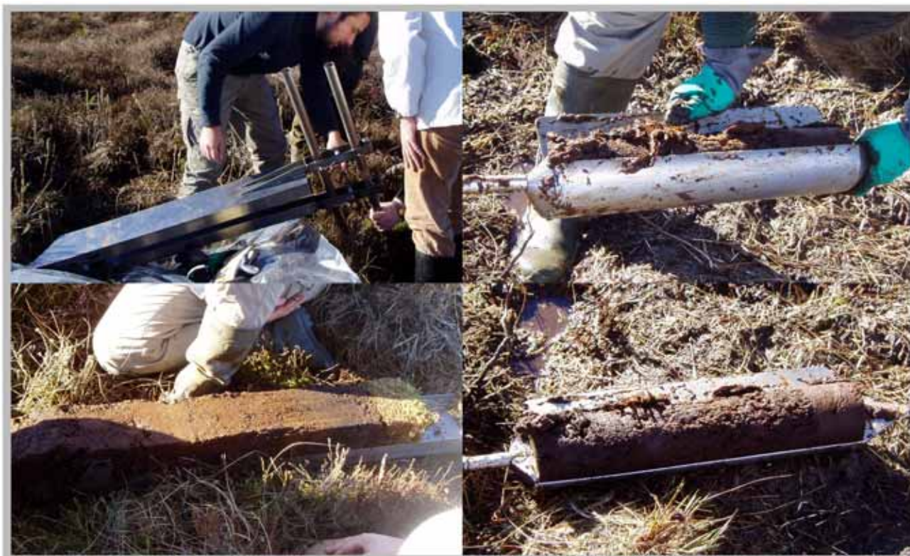
Figure 2. The two main types of corer that are used for sampling peat profiles. On the left, the Wardenaar corer and the peat monolith that can be retrieved with it. On the right, the Russian D-corer and the semi-cylindrical sample that it delivers.
