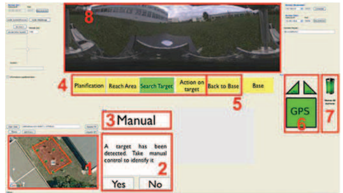
Fig. 1. Ground Station Interface: 1) “tactical map;” 2) “interactive panel,” 3) “mode annunciator;” 4) “synoptic;” 5) “back to base;” 6) “GPS and ultrasound status;” 7) “battery status;” 8) “panoramic video.”
