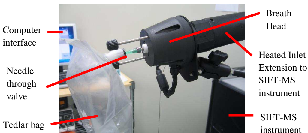
Figure 2-4. Photograph showing a Tedlar bag attached to the Breath Head and Heated Inlet Extension of the SIFT-MS instrument via a needle through the bag's valve.
