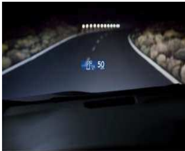
Figure 2.6: Lexus RX 450h head-up display
