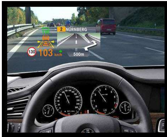
Figure 2.5: BMW head-up display
