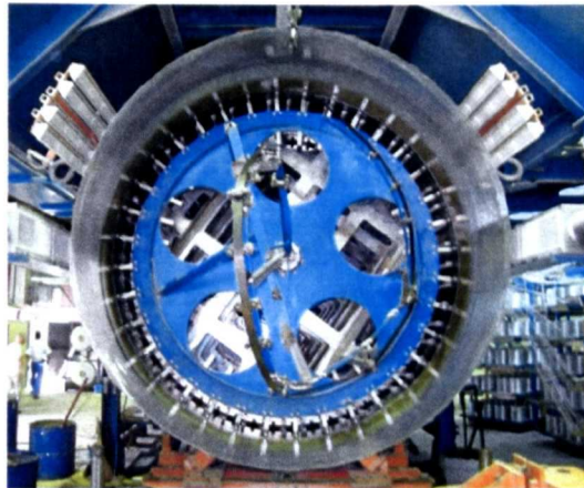
Fig 1-14 Modern fibre winding equipment capable of producing 48m/hr of \text{\O}600\text{mm} GFRP tube
