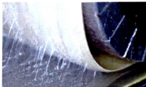
Fig 3-14 Deviation in bending radius from the roller radius during high tack peel
