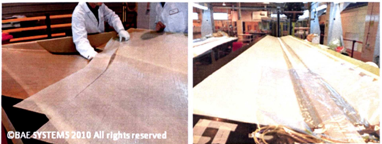
Fig 4-6 Hand finishing of plies (left) to complete 7m blade skin lay-up (right)
