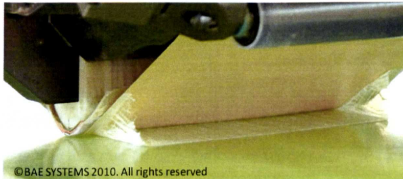
Fig 4-60 ATL lay-up at ambient temperature ( \approx 20^{\circ}\text{C} ) and 4 mm/min feed rate
