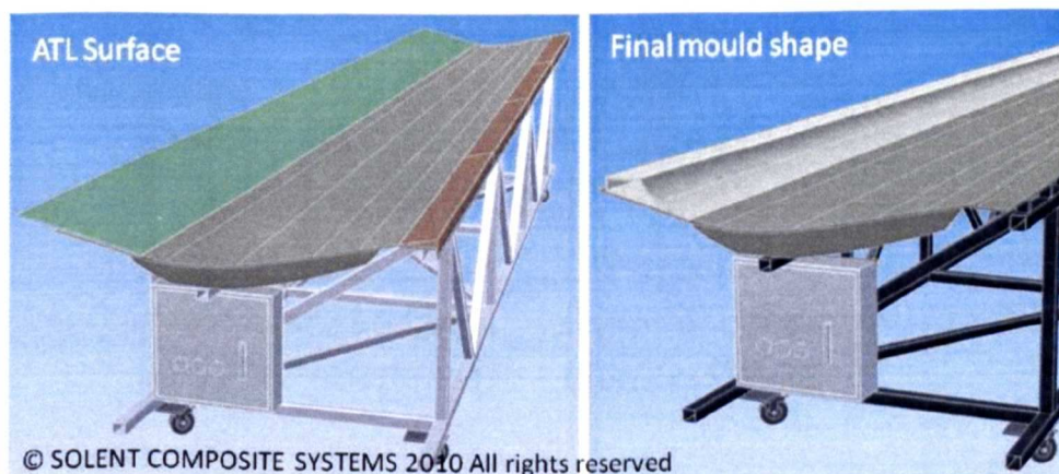
Fig 3-4 Demonstrator moulds with plates to allow ATL lay-up on surfaces below 15° (left), blocks are then inserted to form leading and trailing edges (right)
