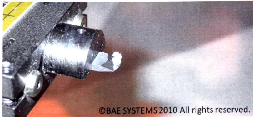
Fig 4-2 Resin build up on Cincinnati V4 blades believed to cause cutting difficulties
