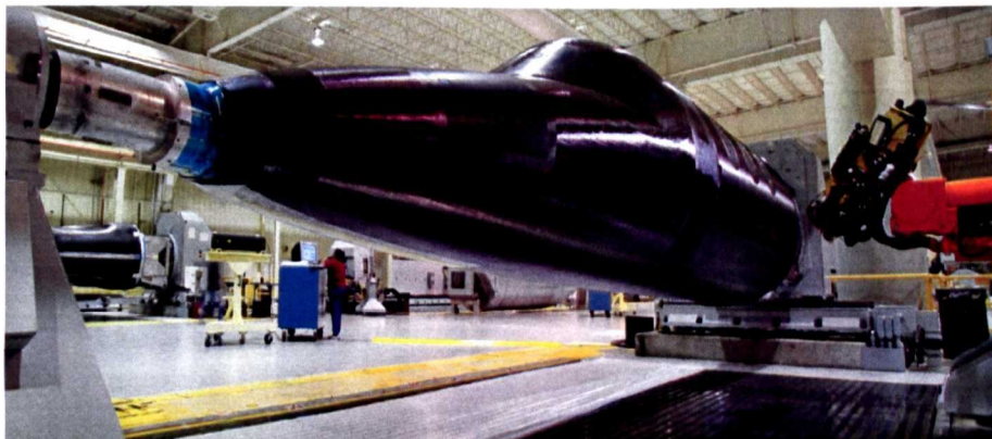
Fig 1-13 Typical automated tape winding process [41]
