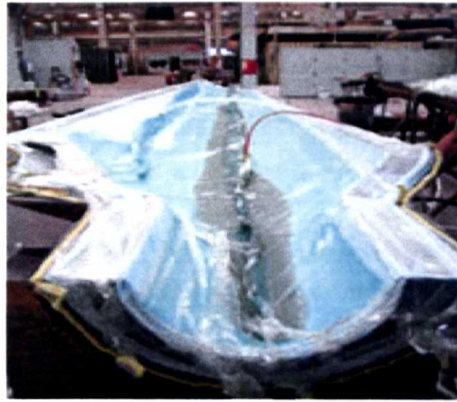
Fig 1-8 Resin impregnation during VI of a turbine blade shell [Tygavac]
