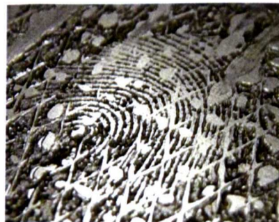
Fig 3-12 Finger print residue on the rigid substrate prior to testing was revealed in resin deposition patterns after peel
