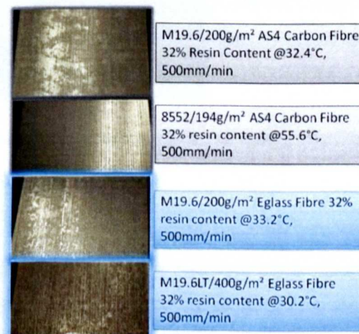
Fig 5-6 A comparison of E-glass and carbon fibre prepreg resin deposition pattern on rigid substrates
