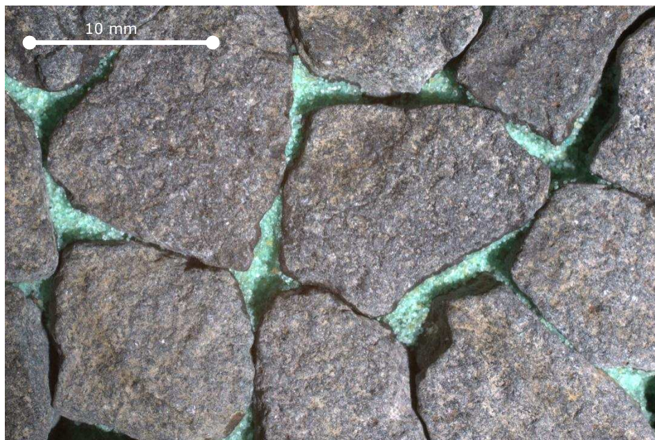
Figure 4.2 Dolerite aggregate specimen prepared for polishing
