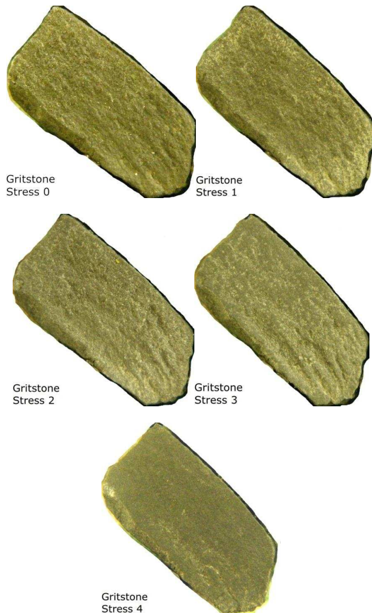
Figure 6.3 Photographs of gritstone particle 1 at each stage of polishing (from compact camera)
