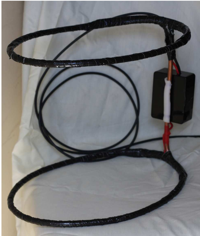
Figure 4.4: Large receiver coil. f = 4.75 MHz, \Delta f = 0.06 MHz, Q = 79 , Dimensions = 36 \times 26 \times 25 cm.
