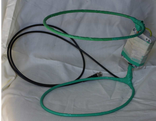
Figure 4.2: Small receiver coil. f = 4.73 MHz, \Delta f = 0.03 MHz, Q = 158 , Dimensions = 26 \times 17 \times 18 cm.
