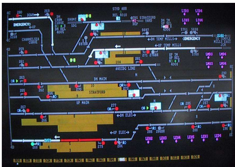
Figure C- 21: IECC Screen View
