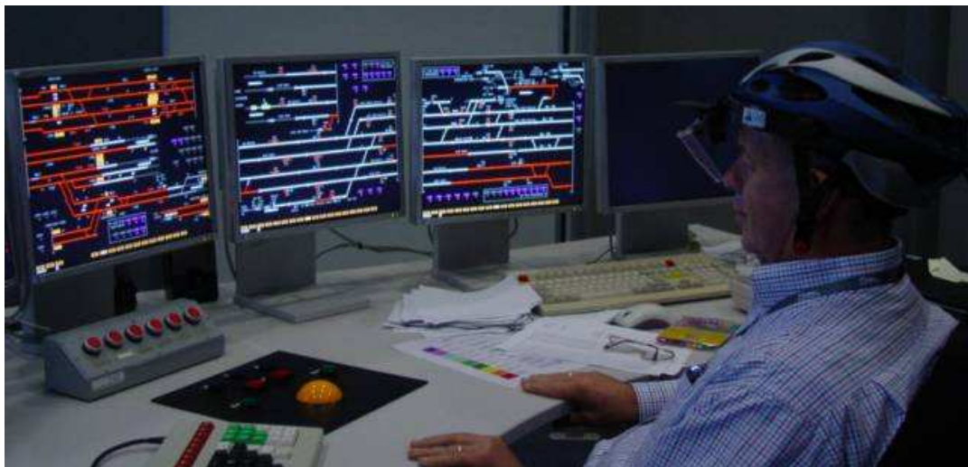
Figure 6-10: Signaller at Simulator with Eye Tracking Helmet
