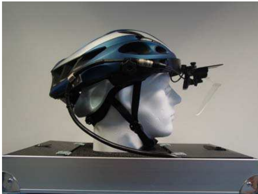
Figure 6-3: Head Mounted Eye Tracker
