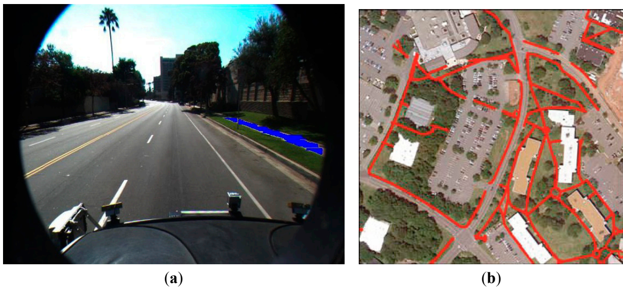
Figure 4. Sidewalk detection techniques: (a) sidewalks detected (blue) in Google Street View; image (b) segments (red) detected as sidewalks.
