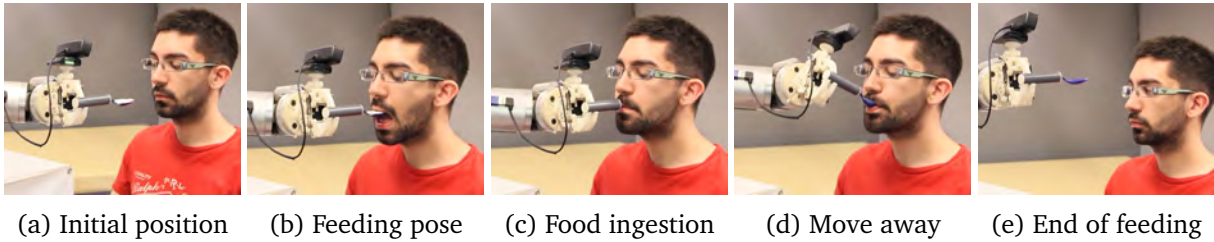
Figure 2.3: Example of a feeding execution for the case of a user with reduced mobility.
