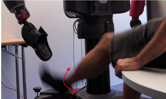
Figure 5.6: Example of user moving the foot. This will trigger an ask action to stop the movement, and may also produce a speed change.
