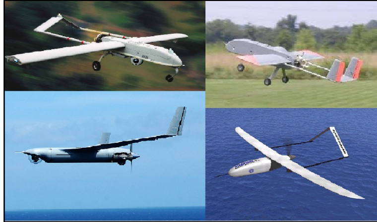
Figure 1-4: Typical LALE UAVs - Clockwise from Upper Left: AAI Shadow200 (Unmanned Systems Technology, 2012), VectorP (Maryland Aerospace, 2015), AAI Aerosonde Mk1 (Courtesy of Aerosonde/AAI), and Boeing/Insitu ScanEagle (Unmanned Systems Technology, 2012)
