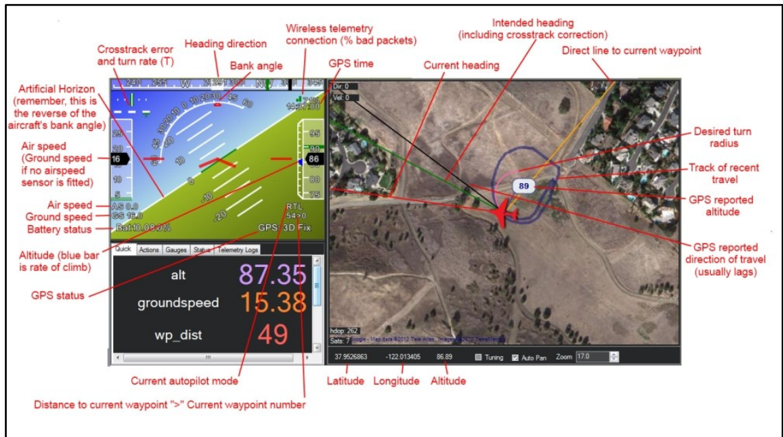
Figure 1-5: APM Mission Planner GCS Display with Annotations (courtesy of 3D Robotics)
