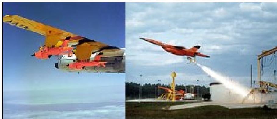
Figure 1-2: Hercules-Launched Ryan Firebee used in Vietnam (USN, Public Domain) (left), and Ryan Teledyne Firebee II Recon UAV using a rocket-assisted launch in 1982 (right). (USAF, Public Domain)
