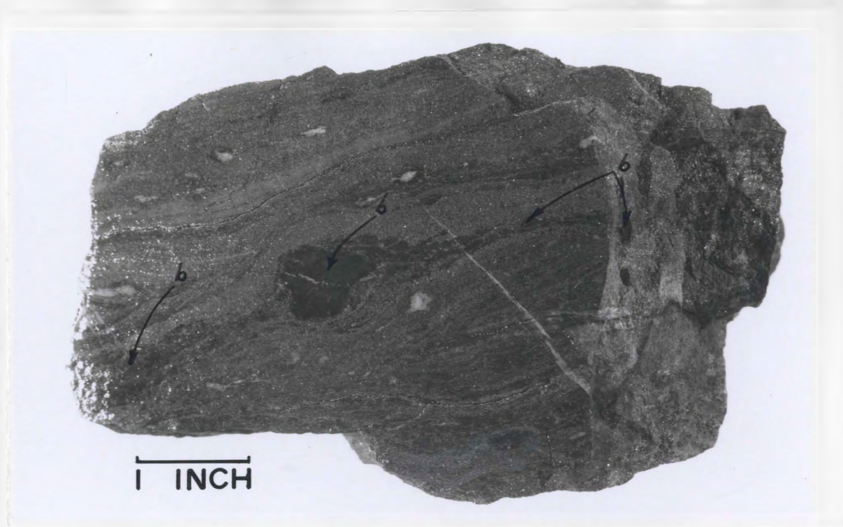
a: Boudinized jasper band in massive banded pyrite ore from Rendell-Jackman showings. Boudins indicated by "b".
