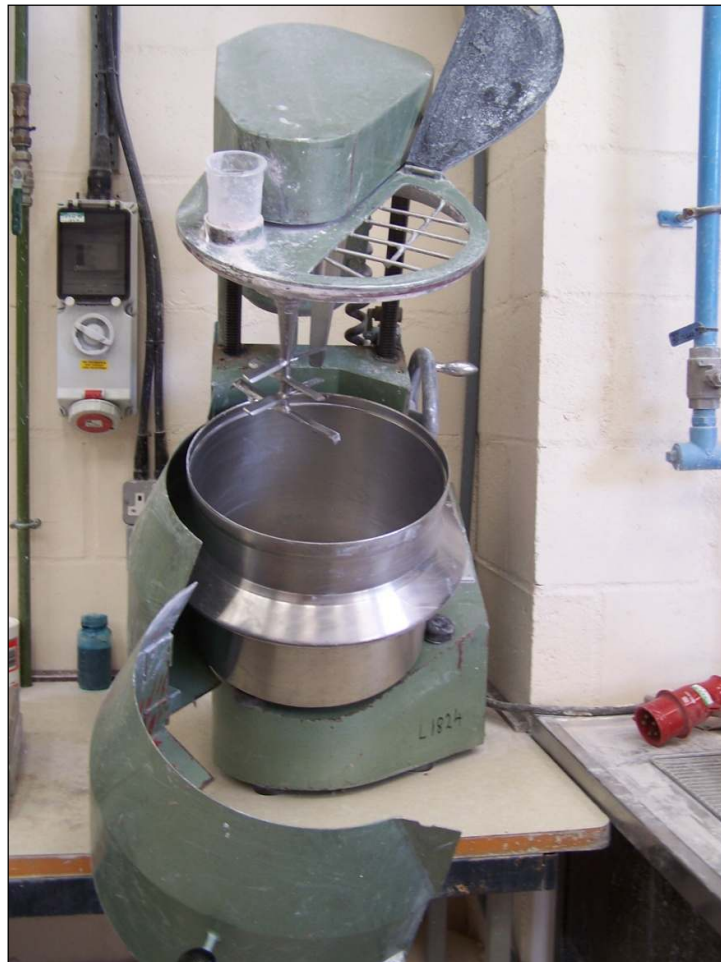
Figure 3-15: Eirich mixer (Maschinenfabrik Gustav Eirich GmbH & Co. KG, Hardheim, Germany) with the mixing blades and bowl visible.
