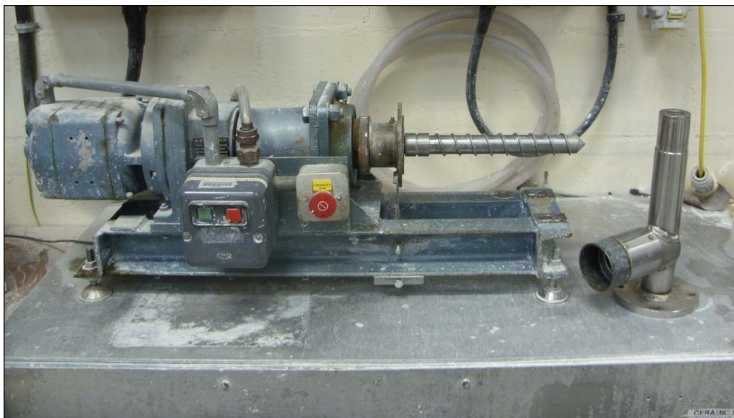
Figure 3-14: Laboratory-scale pug (Imerys Minerals Ltd, Par, UK)
