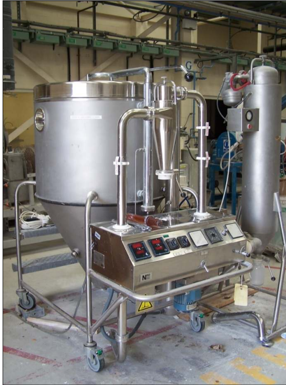
Figure 3-13: Mobile Minor spray drier with a rotary atomiser (GEA Process Engineering Inc, Maryland, US)
