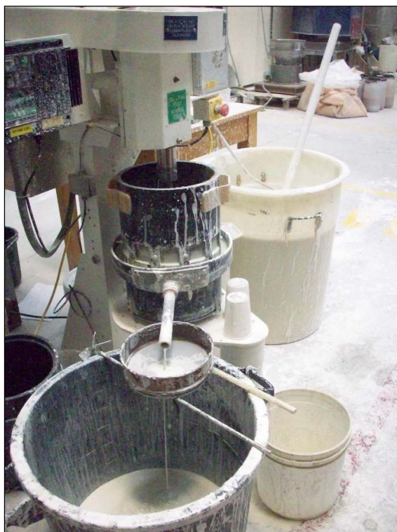
Figure 3-12: Stirred Media Mill Set Up
