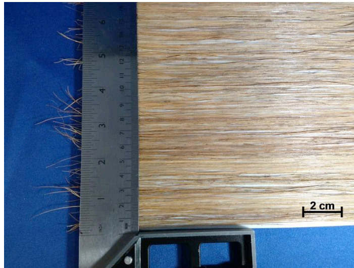
Figure 30 A photograph showing a magnified view of the of manually aligned coir fibre preform.
