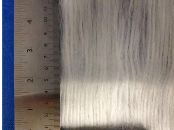
Figure 28 Photograph showing the unidirectional alignment of a bamboo fibre preform obtained via the carding process
