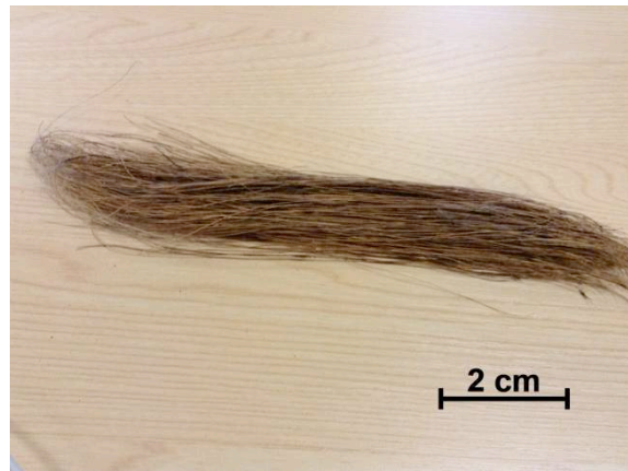
Figure 18 A photograph of as received coir fibres.
