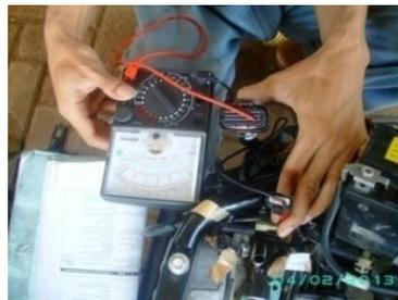
*Gambar 4.1 Memeriksa hubungan kabel hitam/biru antara connector intake air pressure sensor dan connector ECU(Sumber :*
