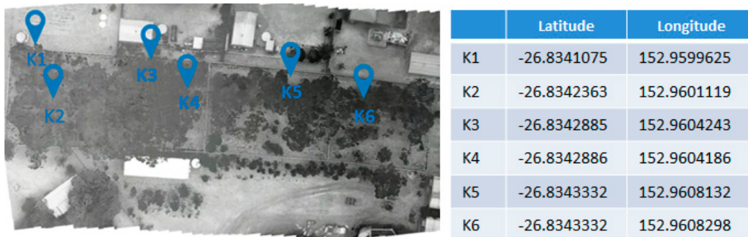
Figure 20. Orthomosaic thermal image with GPS location of detected koalas.
