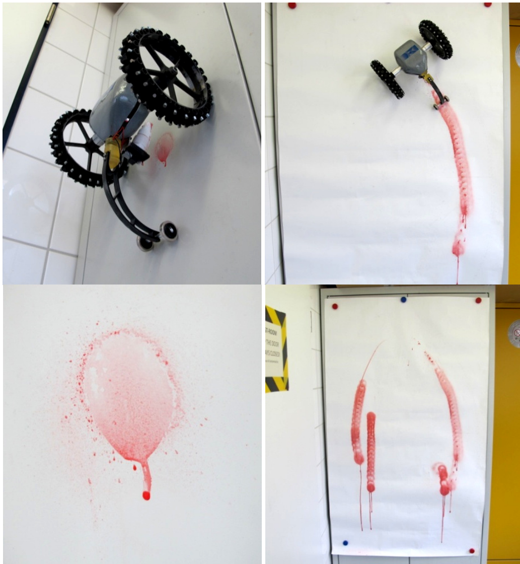
Fig. 12: Experimental results for lightweight crawler and spray unit on a metallic (left) and paper surface (right)
