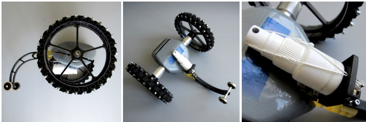
Fig. 11: The lightweight crawler with the marking unit attached
