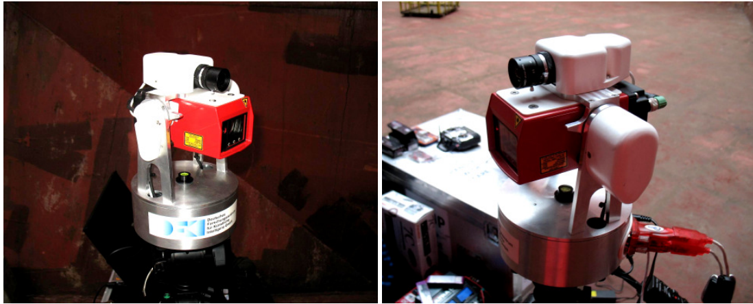
Fig. 3: System overview of the tracking unit that localizes the inspection robot within the vessel. The camera is mounted above the laser range finder and both are actuated with the servo motors situated beneath the covers.
