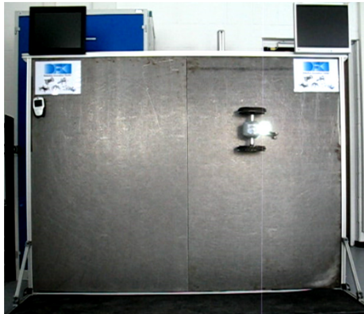
Fig. 5: The DFKI lightweight crawler on the test wall with the tracking LED switched on.
