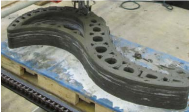
Figure 2 - A concrete printed object: Note the ribbing on the side from the layered approach (Source: Austin, Lim & Le, 2012)
