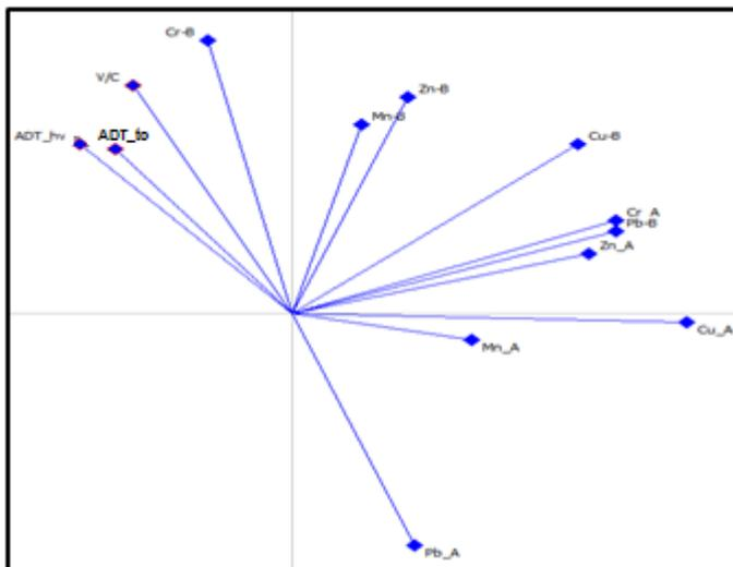
**Fig. 2:** GAIA biplots: (a) Original biplot and (b) Biplot after removing the study sites to improve clarity (Legend: Total traffic volume - ADT\_to; Total heavy duty traffic volume – ADT\_hv; Congestion – V/C; Subscripts B and A correspond to build-up and atmosphere, respectively)
