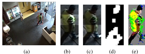
Fig. 3. An image to be searched, and a particle location (red bounding box) are shown in (a). Given this particle location, regions of interest for the torso (b) and legs (c) are defined. Within each of these regions, the motion (d) and colour (e) are considered and used to determine how well the candidate bounding box matches the query (note that when considering the colour, a soft decision approach is used rather than the hard decision indicated by (e)).
