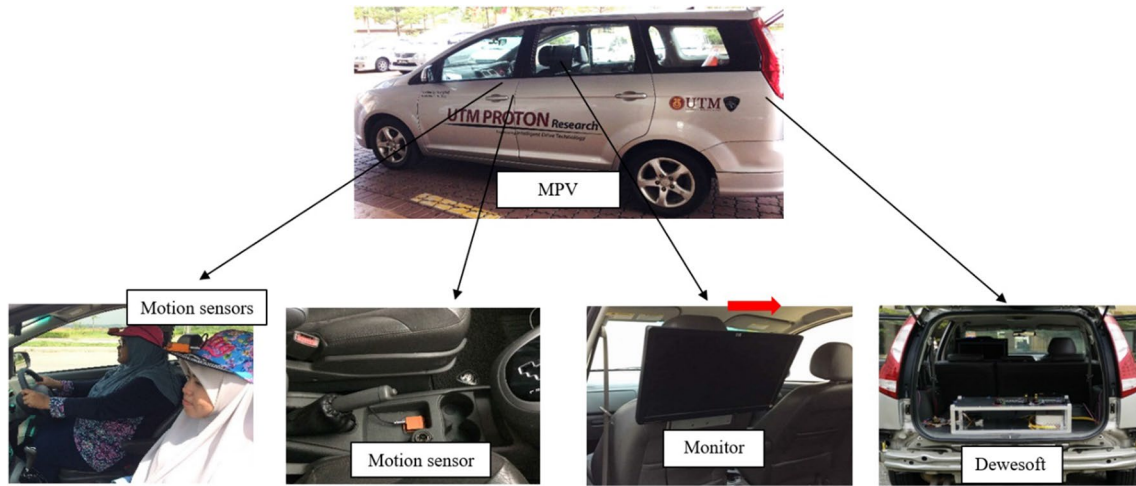
Fig. 5 Location of the equipment during the experiment
