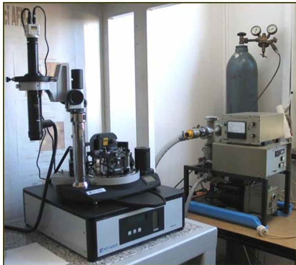
Scanning Probe Microscope SPM Ntegra (NT-MDT)
