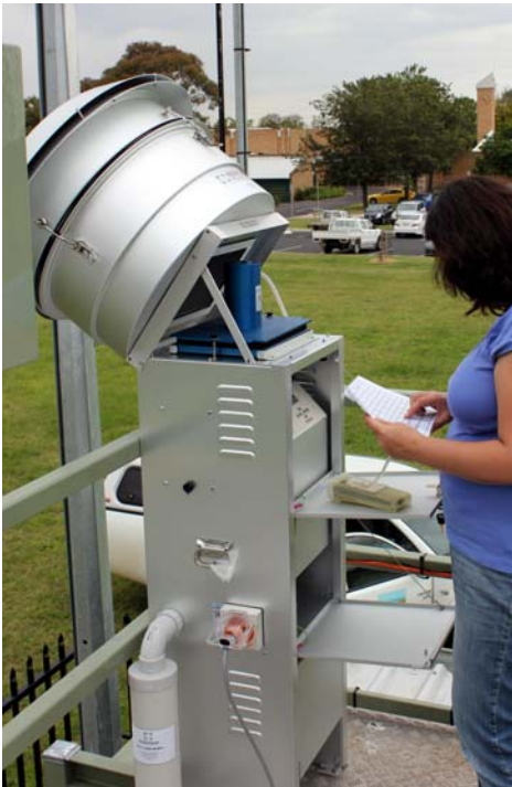
Figure 5 The high volume sampler at Singleton with flow rate calibration being carried out
