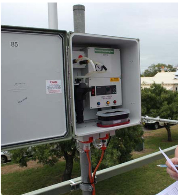
Figure 6 ANSTO ASP sampler with cover open for filter changing
