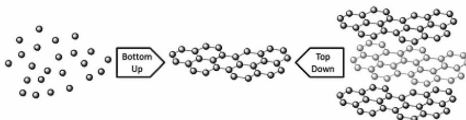
Figure 1.2 Schematic of bottom-up and top-down method of synthesis of graphene. Reprinted with the permission of reference [24]. Copyright 2012 The Royal Society of Chemistry.
