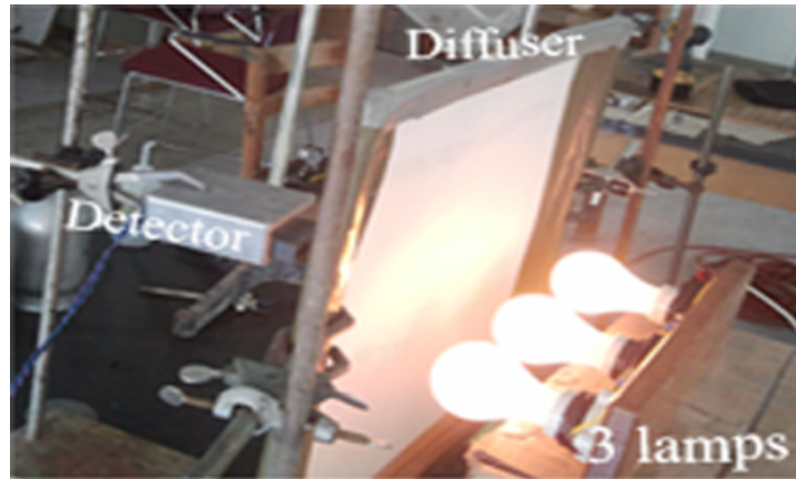
Figure 2.7 Experimental setup for the measurement of radiation from the filament lamp by the two color pyrometer
