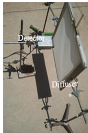
Figure 2.5 Experimental setup for the measurement of sunlight at ~ 12:00 noon. The detector is pointing into the region of diffuser illuminated by the light. The dark patches on the ground are the shadow of detector and diffuser itself and clamps used to hold it. The dark region on the upper part of the diffuser is the shadow of the frame holding it from that side.
