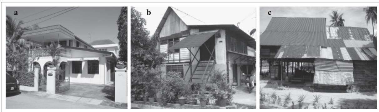
Fig. 1. Building structure in Penang (a) Permanent structure (b) Semi – permanent structure (c) Temporary structure
