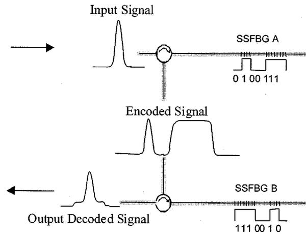
Fig. 1. Outline of the physical approach of pulse encoding and decoding using superstructured fiber Bragg gratings (SSFBGs).
