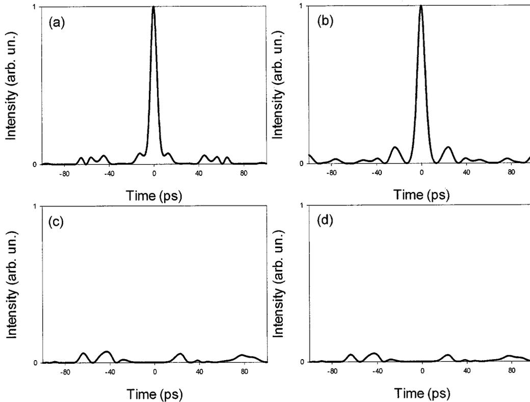
Fig. 6. Calculated traces of the signals after the code:decode process for 2.5-ps soliton input pulses for the grating combinations: (a) G63B-1 : G63B-1\*, (b) G63B-2 : G63B-2\*, (c) G63B-2 : G63B-1\*, and (d) G63B-1 : G63B-2\*.
