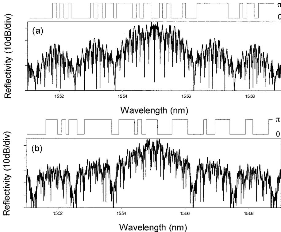
Fig. 5. Superstructure profiles (upper traces) and corresponding calculated reflectivity spectra (lower traces) for (a) G63B-1 and (b) G63B-2.
