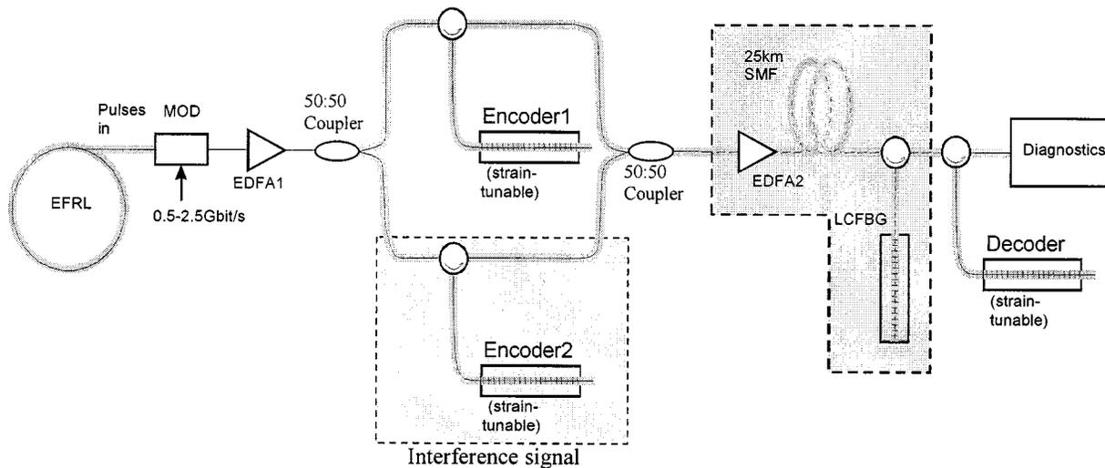
Fig. 7. Experimental setup (EDFA: erbium-doped fiber amplifier; LCFBG: linearly chirped fiber Bragg grating).
