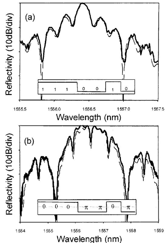
Fig. 8. Reflectivity spectra for (a) the M7U-1 and (b) the M7B-1 grating (solid lines: experimental measurements; dashed lines: theoretical plots).
