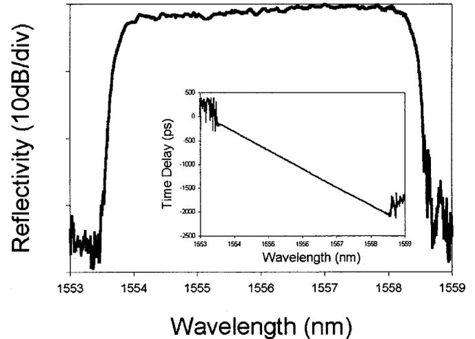
Fig. 15. Reflectivity spectrum of the dispersion-compensating grating. The time delay diagram is shown in the inset.
