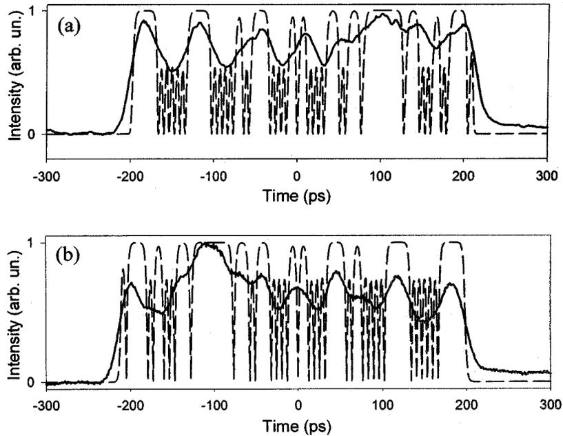
Fig. 11. Traces of the encoded waveforms for (a) the G63B-1 and (b) the G63B-1\* grating, for 2.5-ps soliton input pulses. Solid lines represent experimental measurements, whereas dashed lines represent theoretical plots. The detection bandwidth of the experimental measurement ( $\sim 20$  GHz) was not taken into account for the theoretical calculation.
