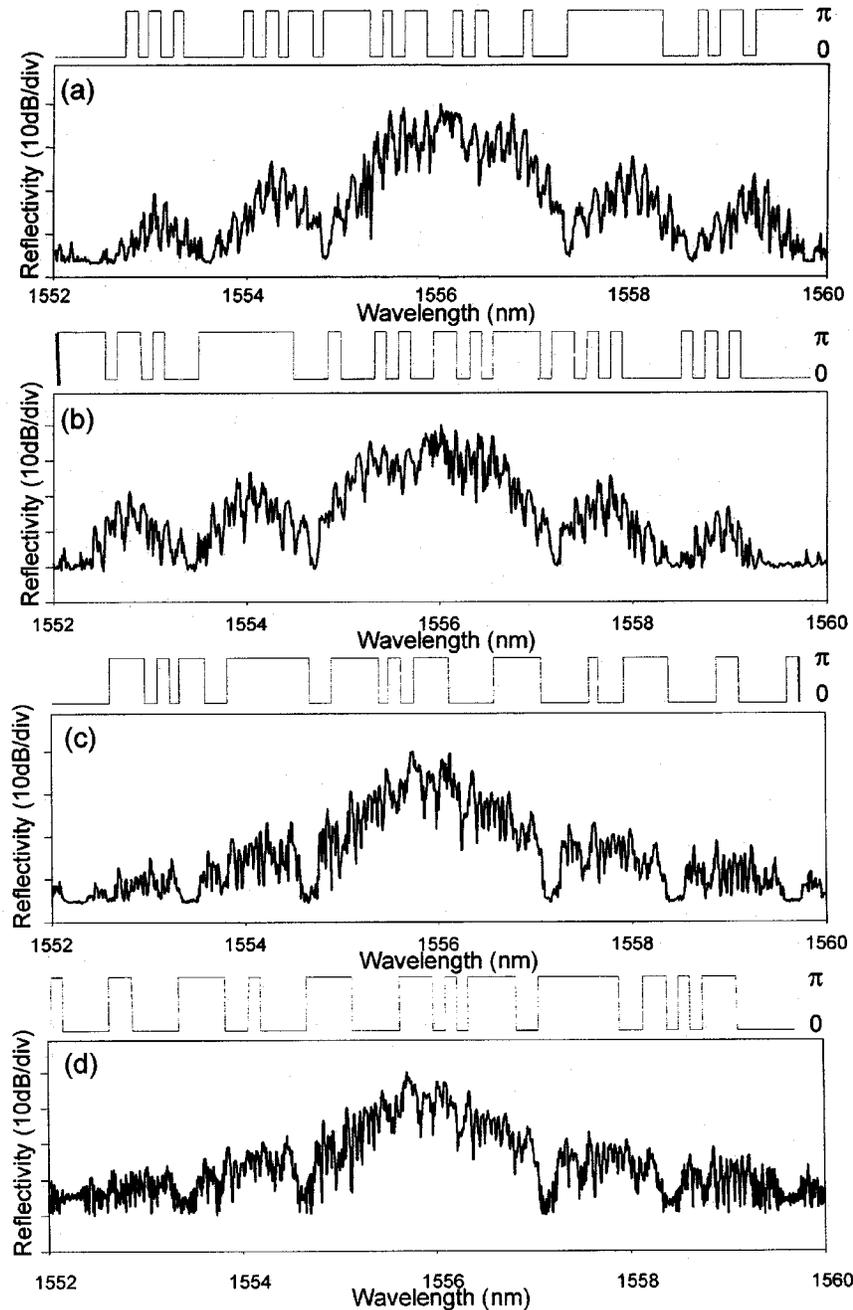
Fig. 9. Superstructure profiles (upper traces) and the corresponding measured reflectivity spectra (lower traces) for (a) G63B-1, (b) G63B-1\*, (c) G63B-2, and (d) G63B-2\*.
