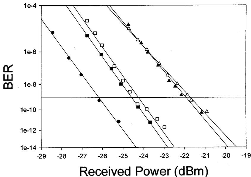
Fig. 17. BER curves for the G63B-1 : G63B-1\* combinations (closed circles: laser back-to-back; closed squares: no transmission; open squares: after transmission; closed triangles: with second channel present and no transmission; open triangles: with second channel present and transmission). The data rate was 1.25 Gb/s.
