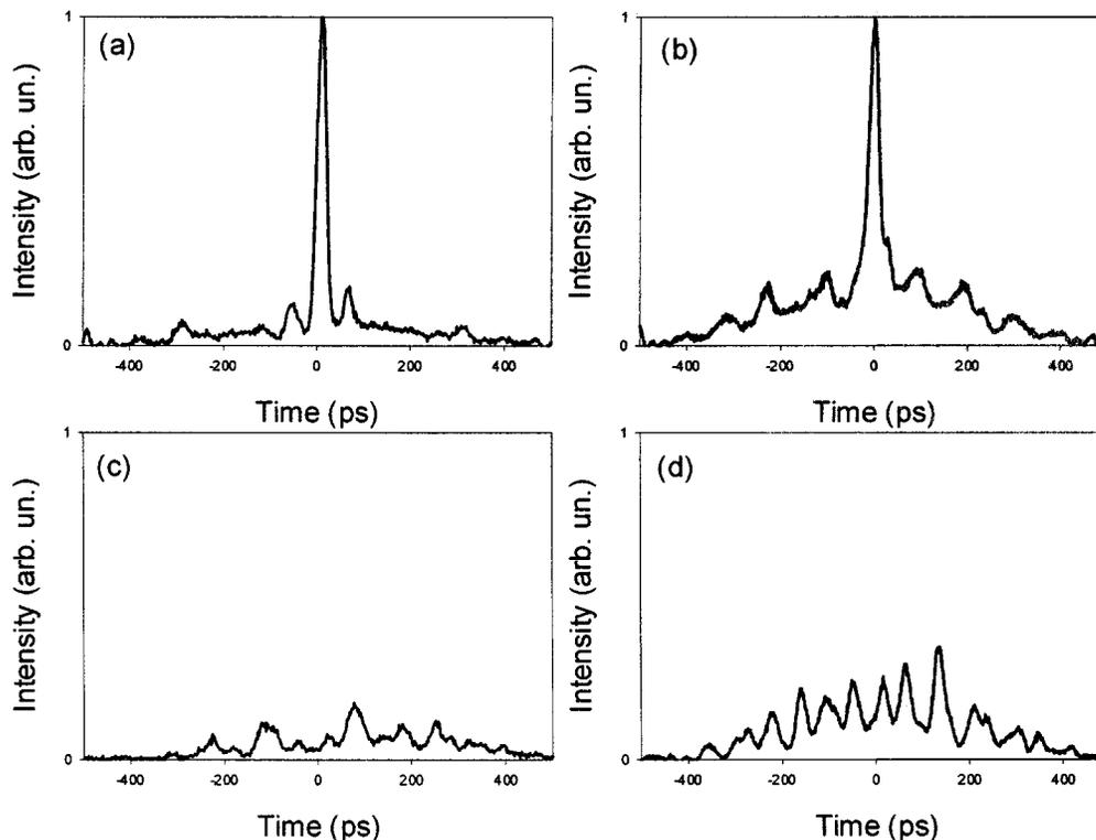
Fig. 13. Traces of the signals after the code:decode process for 2.5-ps soliton input pulses, for the grating combinations: (a) G63B-1:G63B-1\*, (b) G63B-2:G63B-2\*, (c) G63B-2:G63B-1\*, and (d) G63B-1:G63B-2\*. The detection bandwidth was  $\sim 20$  GHz.
