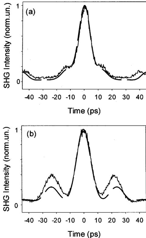
Fig. 14. Intensity SHG autocorrelation traces of the signals after code : decode process for 2.5-ps soliton input pulses for the 63-bit grating combinations: (a) G63B-1:G63B-1\* and (b) G63B-2:G63B-2\*. Solid lines represent experimental measurements, whereas dashed lines represent theoretical plots.
