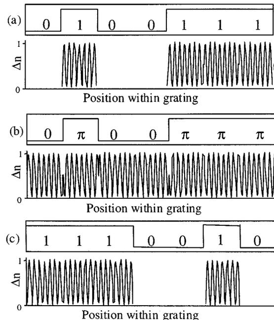
Fig. 2. Schematic examples of temporal codes (upper traces) and corresponding refractive index modulation profiles along the SSFBG structures (lower traces). (a) A unipolar code (M7U-1). (b) A bipolar code (M7B-1). (c) The matched filter to M7U-1 (M7U-1\*). For the cases described in our experiments, the period of the refractive index modulation was  $\Delta \sim 520$  nm and the chip length  $L_{\text{chip}} = 0.66$  mm.
