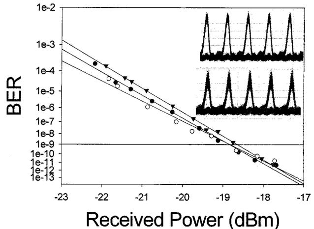
Fig. 16. BER curves for the M7B-1 : M7B-1\* combination (open circles: laser back-to-back; closed circles: decoded signal without transmission; triangles: decoded signal after transmission). Inset shows eye diagrams of the decoded signals without (upper trace) and with transmission (lower trace). The data rate was 10 Gb/s.
