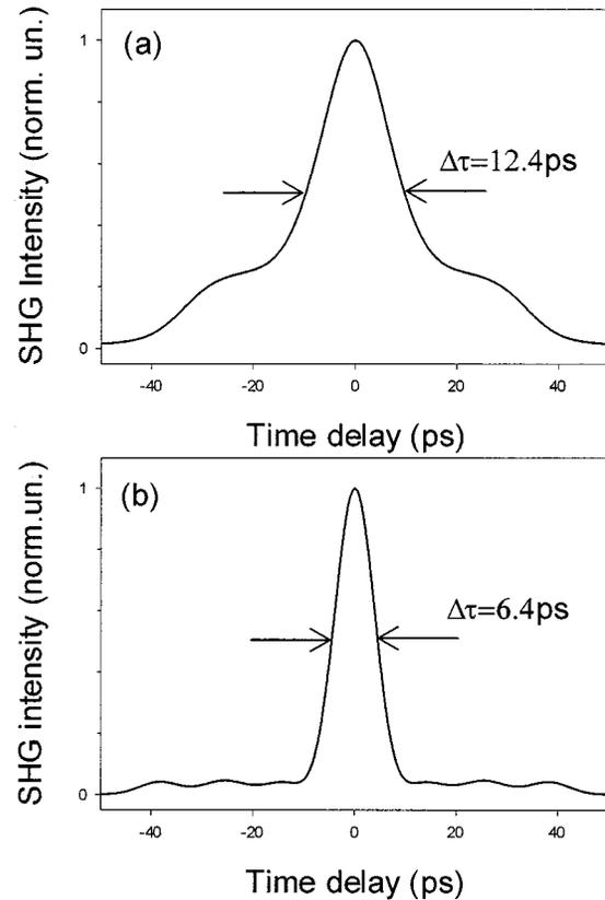
Fig. 4. Calculated traces of the decoded signals for 2.5-ps soliton input pulses for the grating combinations: (a) M7U-1 : M7U-1\* and (b) M7B-1 : M7B-1\*.
