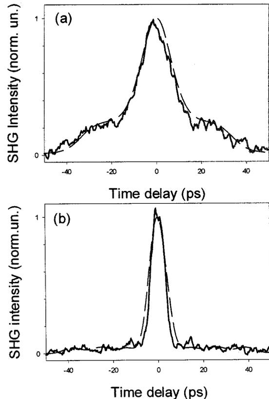
Fig. 12. Intensity SHG autocorrelation traces of the signals after the code:decode process for 2.5-ps soliton input pulses for the grating combinations: (a) M7U-1:M7U-1\* and (b) M7B-1:M7B-1\*. Solid lines represent experimental measurements, whereas dashed lines represent theoretical plots.
