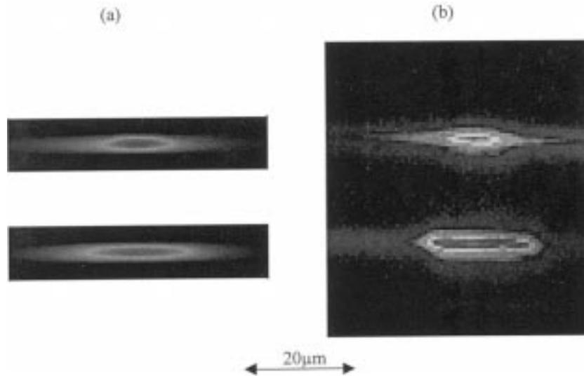
Fig. 5. (a) Calculated and (b) experimentally observed mode profiles for the 8- $\mu\text{m}$  (upper) and 20- $\mu\text{m}$  (lower) ion-milled channel waveguides.
