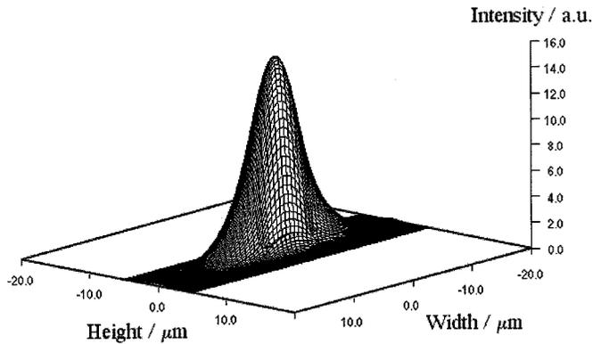
Fig. 6. Calculated mode profile for the 8- $\mu\text{m}$  ion-milled waveguide at a wavelength of 5  $\mu\text{m}$ .
