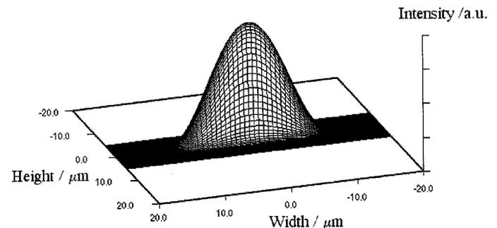
Fig. 8. Theoretical fundamental guided mode for the 20- $\mu\text{m}$ -wide BCB slab loaded channel waveguide at 1.06  $\mu\text{m}$ .
