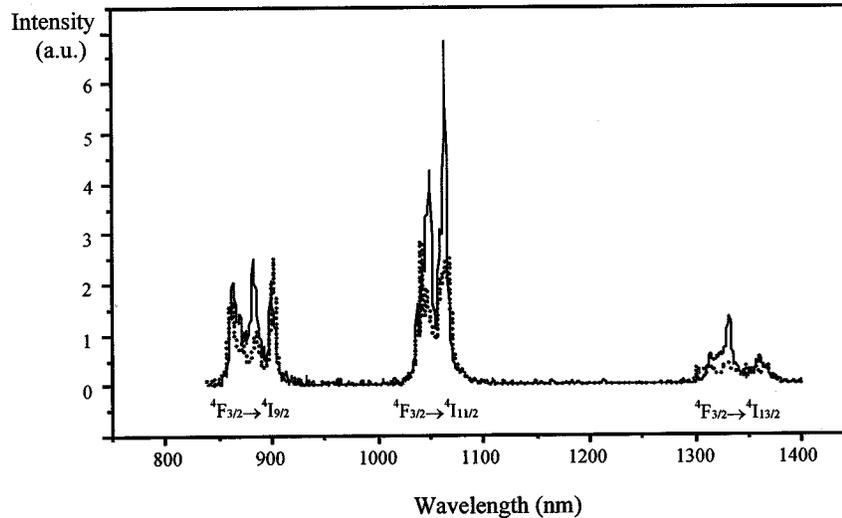
Fig. 2. Polarized emission spectra at 300 K for a 1 at.% Nd:LaF<sub>3</sub> thin film. (Line:  $\pi$  polarization. Dots:  $\sigma$  polarization.)
