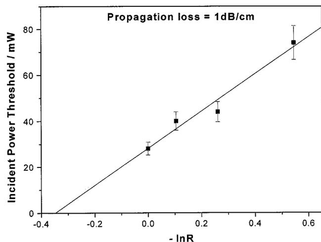
Fig. 10. Plot of incident power threshold against  $-\ln R$  for the  $8\text{-}\mu\text{m}$ -wide ion-milled channel waveguide.
