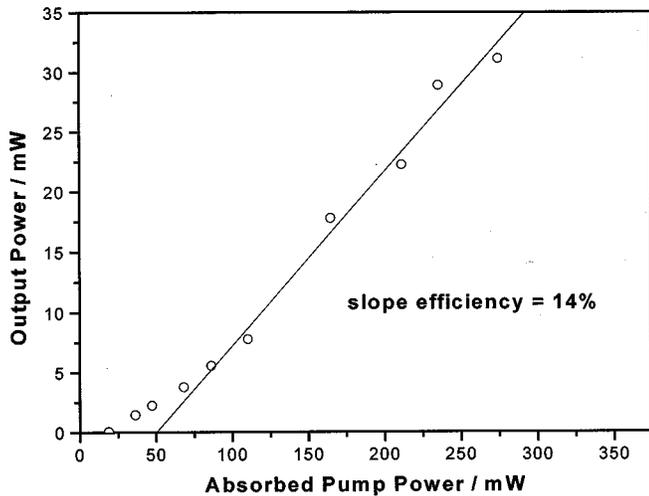
Fig. 11. Output power against absorbed pump power for the 20- $\mu$ m-wide BCB channel waveguide.
