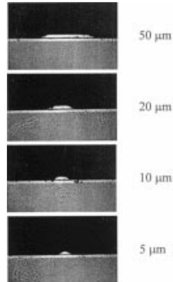
Fig. 7. Microscope pictures of the polished end-face of the BCB channel waveguides of various widths.
