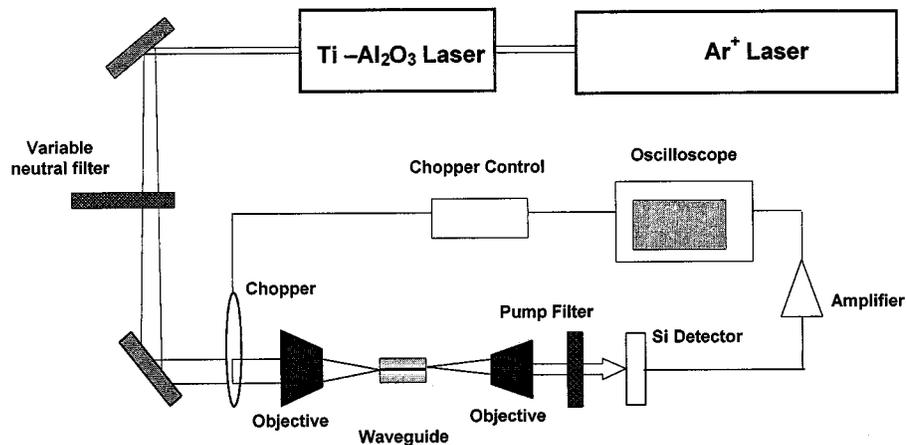
Fig. 9. Experimental arrangement for waveguide laser characterization.
