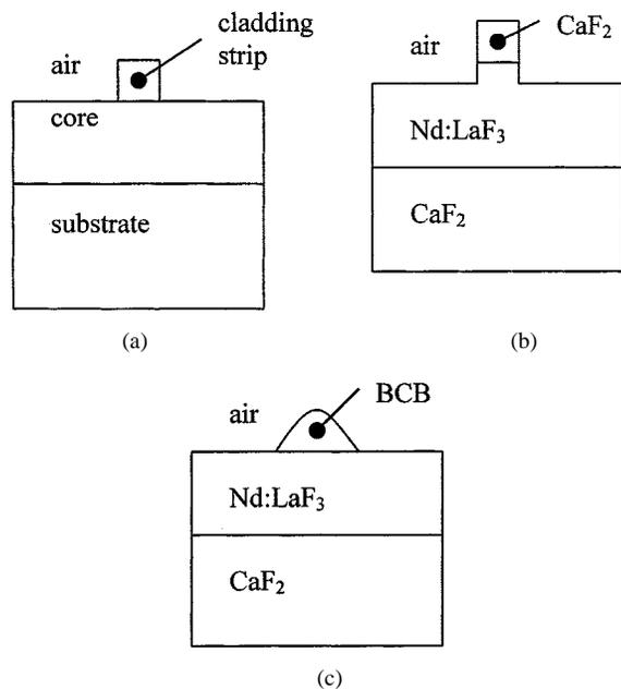
Fig. 4. Channel-waveguide geometries. (a) Standard slab loaded geometry. (b) Ion-milled channel waveguide. (c) Polymer overlay channel waveguide.
