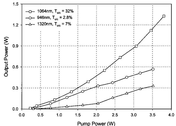
Fig. 4. Plot of the diode-pumped waveguide laser output power versus incident pump power for three transitions in Nd:YAG.
