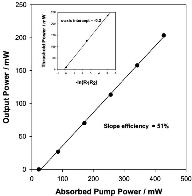
Fig. 2. Plot of output power versus absorbed pump power for the Ti:sapphire-pumped waveguide laser. Inset, plot of threshold incident pump power versus output coupling.
