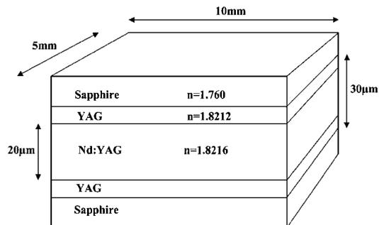
Fig. 1. Schematic of the double-clad waveguide geometry.
