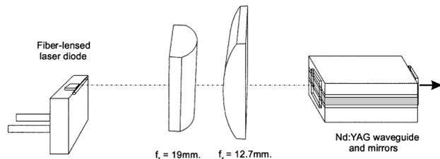
Fig. 3. Schematic diagram of the diode end-pumping arrangement.
