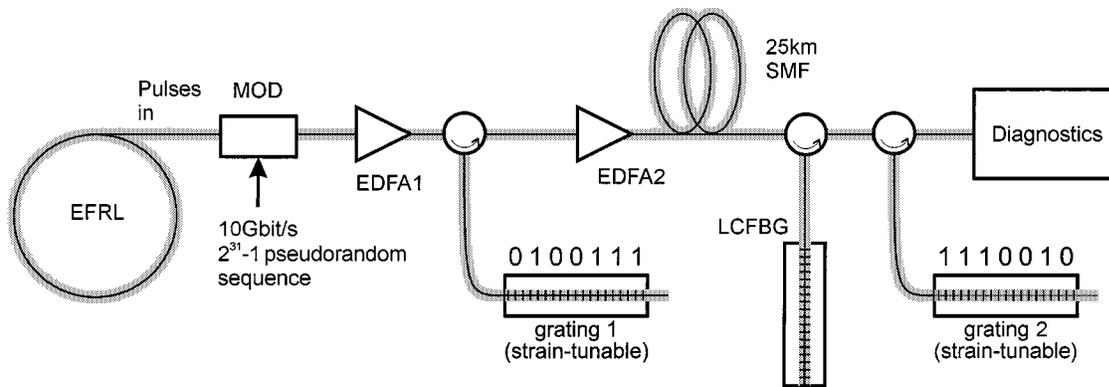
Fig. 1. Experimental setup (MOD: LiNbO<sub>3</sub> electrooptic modulator; EDFA: Erbium-doped fiber amplifier; SMF: single-mode fiber).
