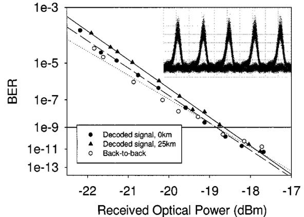
Fig. 5. BER measurements of the decoded signal before and after transmission. Inset: Eye diagram of the decoded signal after transmission.
