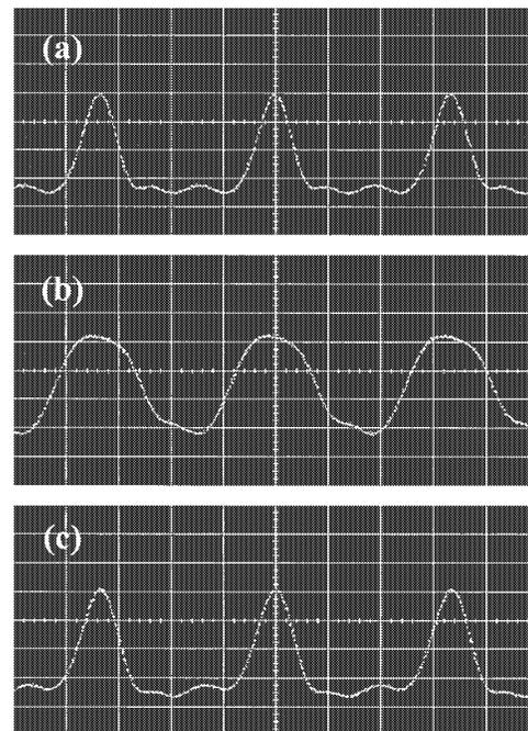
Fig. 3. Oscilloscope traces of (a) incoming 2-ps pulse stream (b) encoded pulses, and (c) decoded pulses (detection bandwidth:  $\sim 20$  GHz–30 ps/div).
