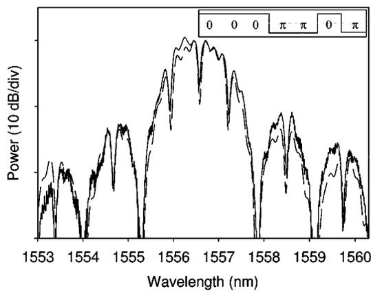
Fig. 2. Spectral response of the 7-chip 160 Gchip/s bipolar encoding SSFBG (solid line: measured response, dashed line: designed response). Inset: bipolar code.
