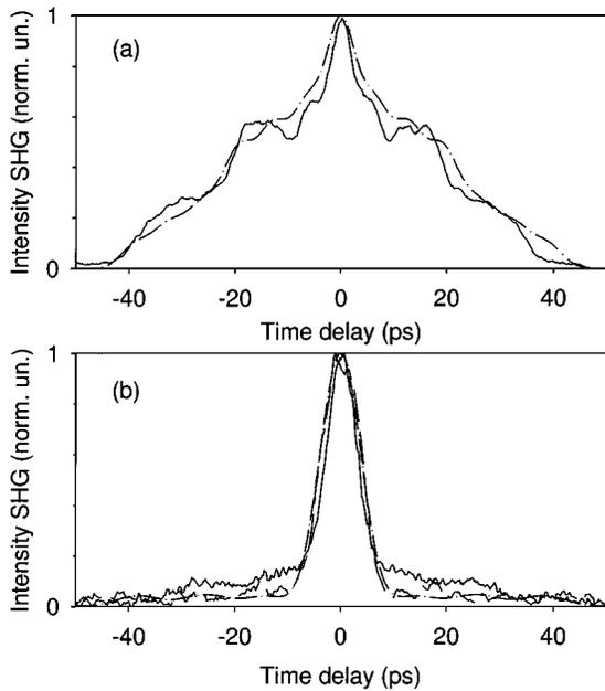
Fig. 4. Intensity autocorrelation functions of (a) the encoded waveforms, and (b) the decoded signals before (dashed line) and after transmission (solid line); the theoretical intensity autocorrelation traces are also shown (dash-dot lines).
