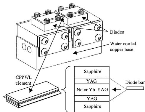
Fig. 1. Schematic drawing of our CPPWL system. The laser is pumped by two laser diode bars located within  $\sim 10 \mu\text{m}$  of either side of the WS. All components are mounted upon a copper base plate that is water cooled.
